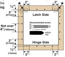
At the latch side only, a screw should be fitted in line with the edge of the frame. It will go through the steel corner brackets. If multiple latches, place fasteners through the base of all latch brackets. Use extra screws on the latch side.
