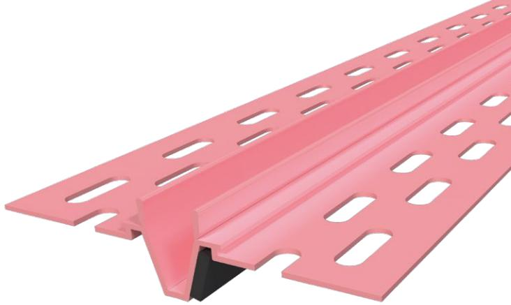
**Advantages:** Made from rust proof, dent resistant PVC to reduce jobsite and handling damage. Does not contain cellulose, a potential food source for mold. Intumescent tape expands when exposed to flame for increased fire protection.
