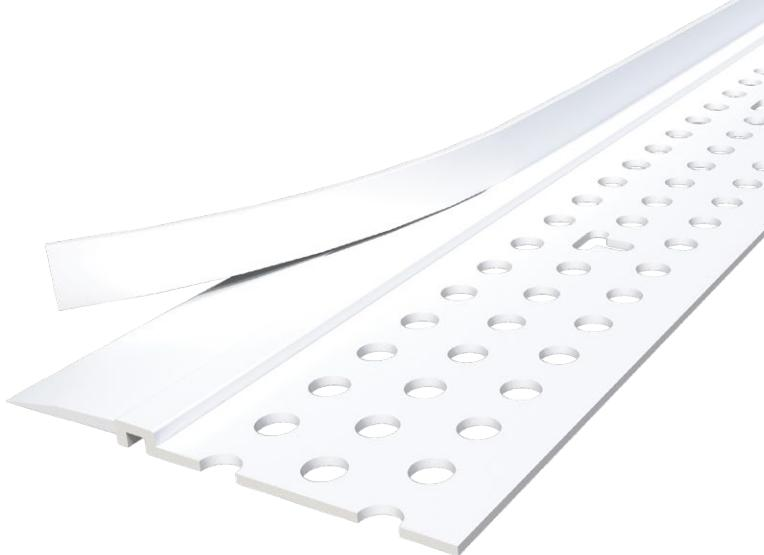
**Description:** Trim-Tex Flat Deflection Bead is designed to prevent inside corner cracking when installed against a ceiling or concrete deck that may be subject to up to  $\frac{1}{2}$ " movement.
