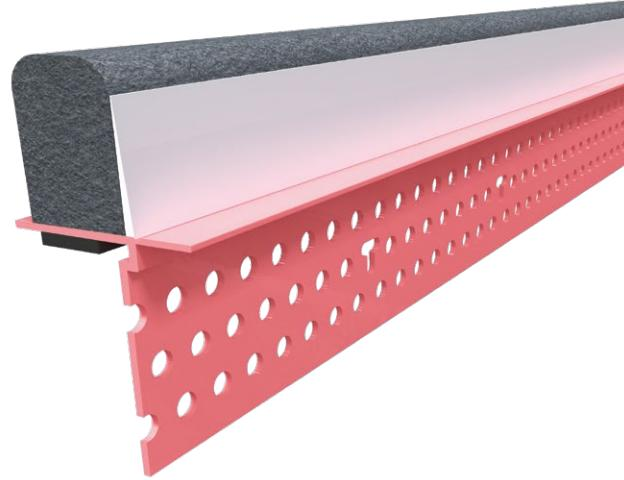
**Description:** Hotrod XL is a fire rated wall mount deflection bead that provides 1- and 2-hour fire ratings for both dynamic and static joints for both fluted deck and concrete assemblies according to UL-2079 5th Edition (for both standard walls and shaft walls) and no spray is required over mineral wool, and is sound tested according to ASTM E90. Sound Reports available upon request. Hotrod XL provides a full  $\frac{3}{4}$ " of building movement.
