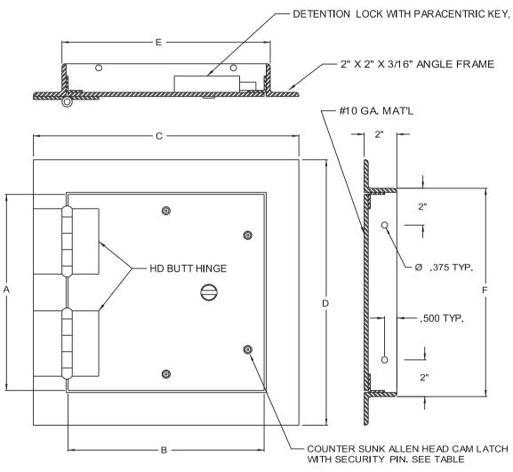
STANDARD FEATURES: DETENTION TYPE DEADBOLT LOCK WITH PARACENTRIC KEY, CARBON STEEL,
