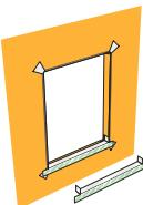
**Sill:** Cut a strip of ExoAir 110AT 6" longer than the length of the sill's opening. For example, a 36" sill will require a 42" strip of ExoAir 110AT. Fold the strip in half lengthwise. Make a 3" cut along the fold at each end so that you have two flaps. This will allow the sheet to be easily positioned into the rough opening and on to the exterior face of the panel.
