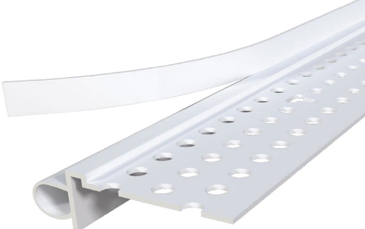
**Description:** Trim-Tex Super Seal Tear Away L Bead is designed to seal around windows, doors, and where drywall butts up to a concrete wall. Gasket compresses upon installation to form a permanent seal that reduces sound transmission, replaces caulk, and provides structural relief at the panel perimeter.
