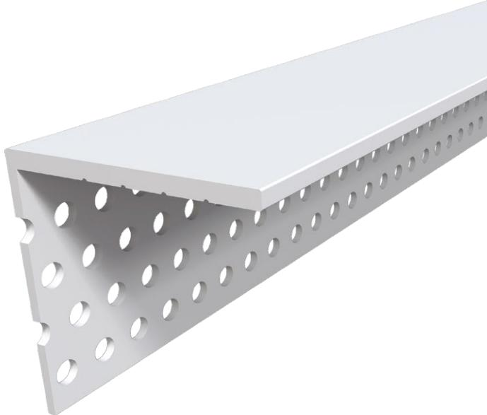
**Description:** Trim-Tex Truss Backing Angle is designed to eliminate inside ceiling corner cracking due to truss uplift of interior partition walls.
